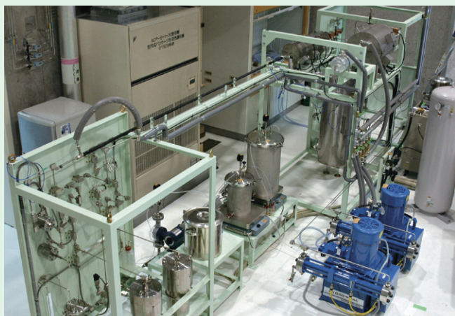
Fig. 2 : Experimental plant based on a continuous reactor using high-pressure supercritical water
