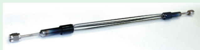
Fig. 1 : High-temperature, high-pressure microreactor and heat exchanger operated at 600°C and 300 MPa
