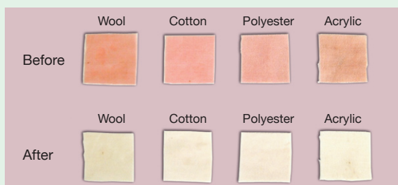
Fig. 2 : Results of CO 2 cleaning of different fabrics stained with fluid paraffin and oil red dye under dual solvent supply
