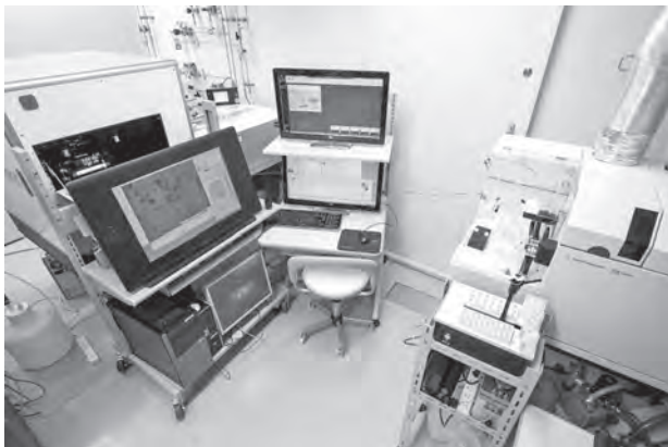
Fig. 5 Laser ablation inductively coupled plasma mass spectrometer (LA-ICPMS). Laser light source by Cyber Laser Inc., ICPMS by Agilent Technologies Japan, Ltd., and other parts were assembled in house.
