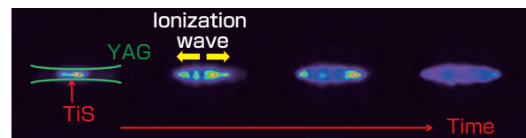
Fig. 15 Temporal breakdown process with initial electron supply
