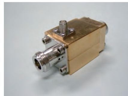
Fig. 13 Inside of a thin-film thermal converter device (top), appearance of a thin-film thermal converter device (middle) and a metal housing for a thermal converter (bottom)
