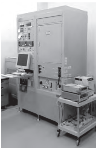
Fig. 7 The apparatus of national standard for thermal diffusivity
