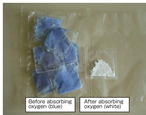
Photo 7. \text{TiO}_2 deoxidant before absorbing oxygen (blue) and after absorption (white).
