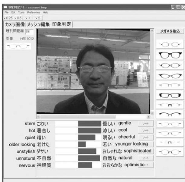
Fig. 10 Style recommendation system for eyeglass frames based on Kansei (sensibility) modeling.
