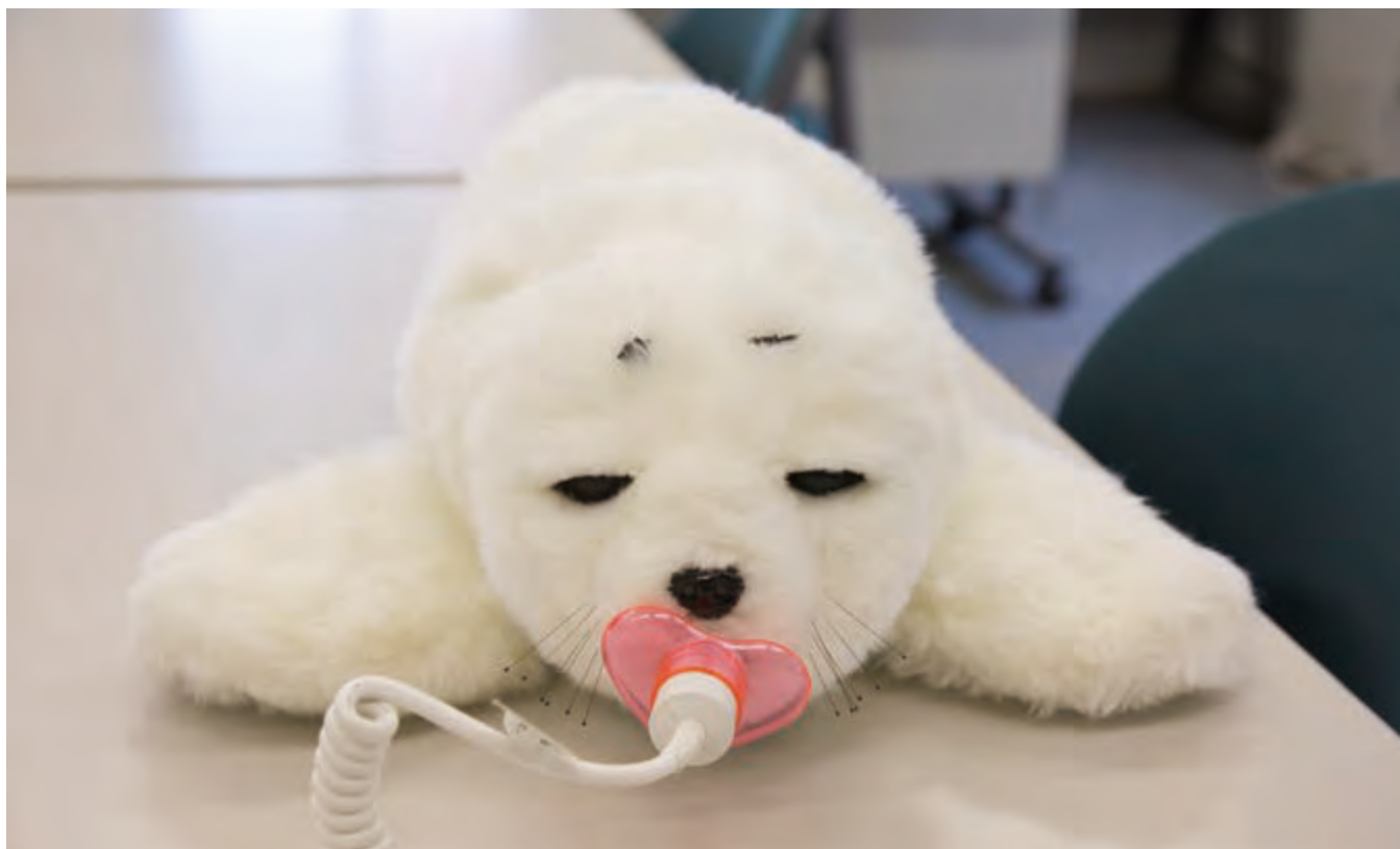
▲ The charger resembles a pacifier. The energy saving design allows the dedicated battery to store enough power for PARO to function for 5–8 hours on a single charge.
