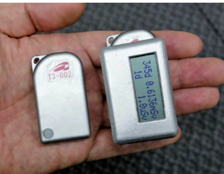
A compact dosimeter that can operate with the same battery for over a year (left) and a display unit (right). As well as pockets, the dosimeter can be put into a child's nametag.
