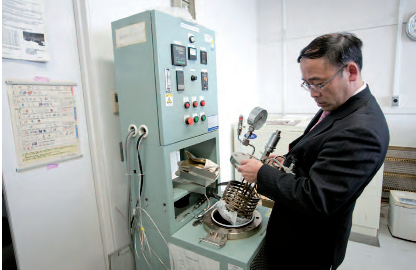
▲ Clay synthesis. Clay synthesized in a pressure vessel is used to fabricate a transparent film.
