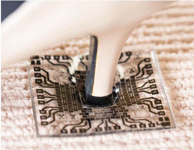
The new transistor being stepped on by a high heel. Because the entire transistor deforms as a single body, performance does not deteriorate even though strong pressure is applied
