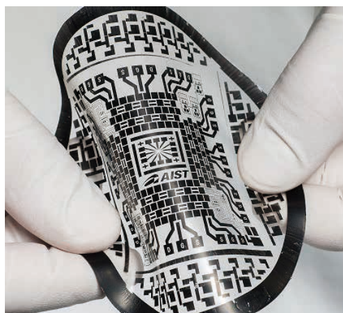
Made completely of materials that can be flexed and stretched, including electrode insulation layers and the substrate
