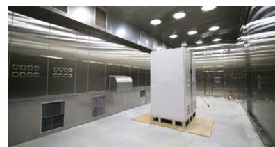
Constant-temperature and -humidity tank in the environmental test chamber
