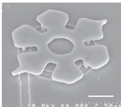
Figure 3: An electron micrograph (scale bar, 5 \mu\text{m} ) of a rotary micromotor driven by Mycoplasma mobile . (Reproduced from Proc. Natl. Acad. Sci. USA 103: 13618-13623 (2006)) Actual rotational movement can be seen at http://www.pnas.org/cgi/content/full/0604122103/DC1#M1 .
