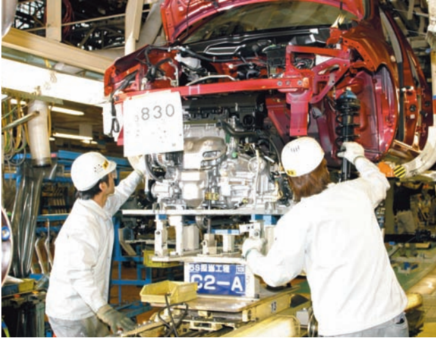
Photo 2 Installing an engine unit
