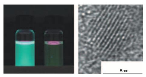
Fig. 3 ZnS/CdSe/ZnS nanoparticles (the left bottle) exhibit fluorescence at 480 nm with several dozen times stronger intensity than that of conventional CdSe/ZnS nanoparticles (the right bottle). The TEM image depicts the size of ZnS/CdSe/ZnS nanoparticles: ca. 5 nm diameter.
