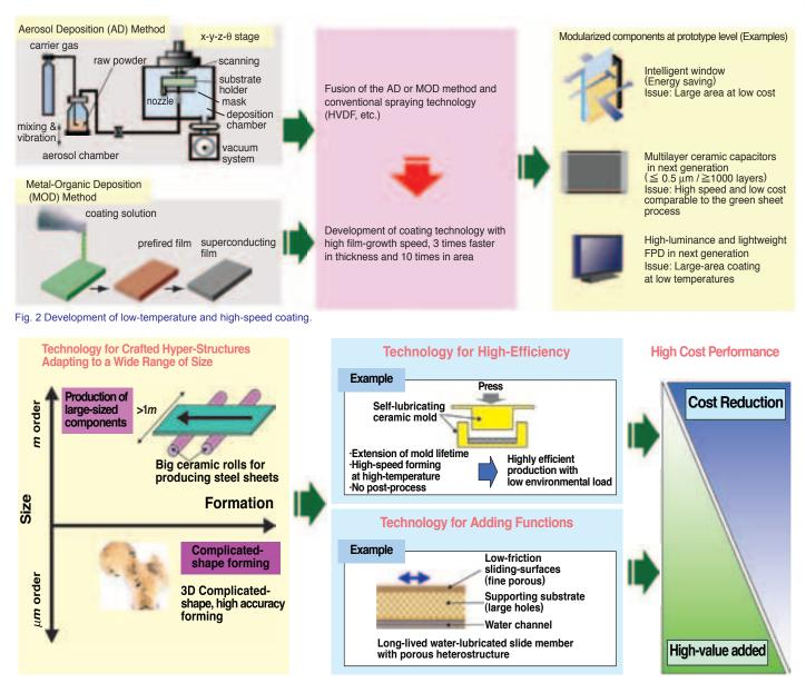
Fig. 3 Development of tailored manufacturing process.
