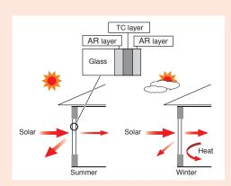
Schematic structure and performance of the window.
