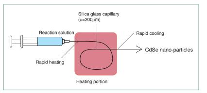
Fig. 1 Schematic diagram showing CdSe nanoparticle synthesis using the microreactor.
