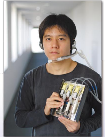
Wearable type olfactory display (provided by Research Center for Advanced Science and Technology of Tokyo University)
