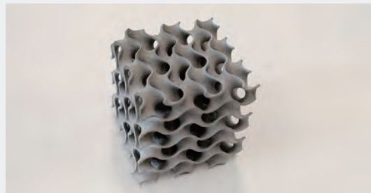
High heat dissipation-shaped metal component formed by metal 3D printer
