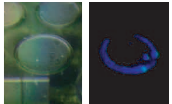
Fig.2 Diamond UV-LED (left) and UV light emission by current injection (right). Blue light can be seen at the same time as UV light emission.
