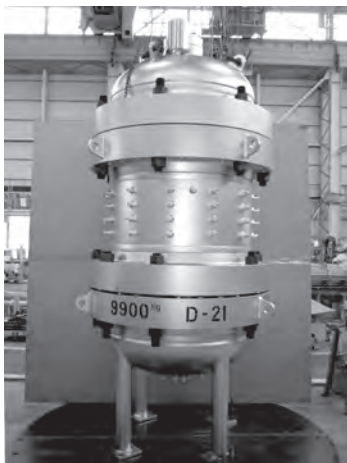
(a) High-pressure vessel of the large-scale laboratory reactor
