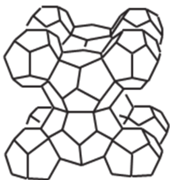
Fig. 1 Crystalline structure of methane hydrate
