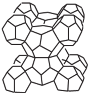
Fig. 1 Crystalline structure of methane hydrate
