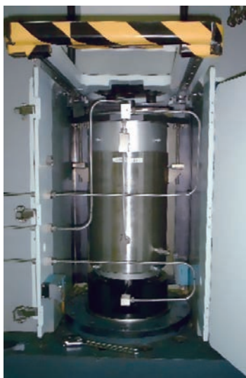
Fig. 8 The pressure vessel, which contains the sample, to be installed in the materials testing device Pressure (confining pressure) is applied to the rock sample in the pressure vessel during the test to replicate the conditions underground.
