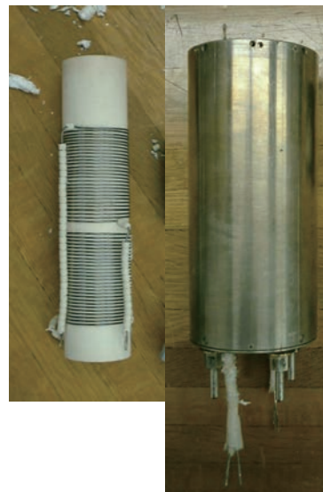
Fig. 9 The heater (electric heating element) developed at AIST
