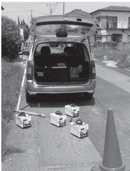
Fig. 2 Measurement using a miniature array with a radius of 0.6 m [Fig. 1(b)]
