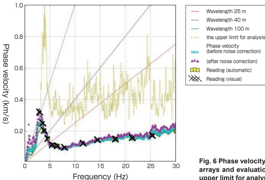
**Fig. 6 Phase velocity (dispersion curve) by miniature arrays and evaluation of automatic reading and the upper limit for analysis**
