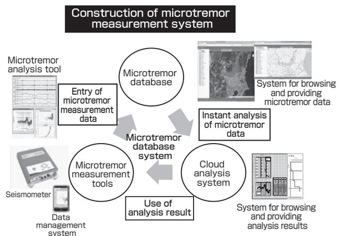
**Fig. 5 Conceptual diagram of microtremor system configuration**
