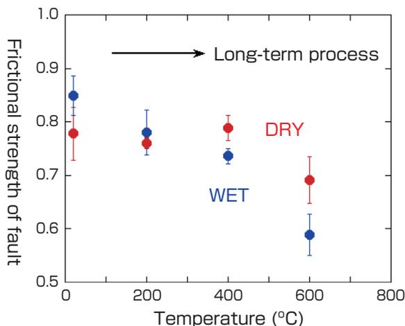
**Fig. 13 Temperature dependency of the frictional strength of the fault plane in rock samples<sup>[18]</sup>**
