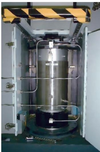
**Fig. 8 The pressure vessel, which contains the sample, to be installed in the materials testing device**
