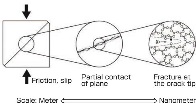
**Fig. 5 Schematic diagram of friction and fractures**
