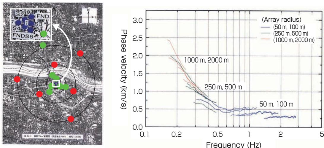
**Fig. 3 Microtremor arrays in conventional exploration (left) and an example of the dispersion curve obtained for each array (right) (after Report [12] of the Tokyo Metropolitan Government)**
