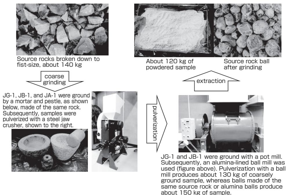
**Fig. 6 Schematics of sample grinding process**
