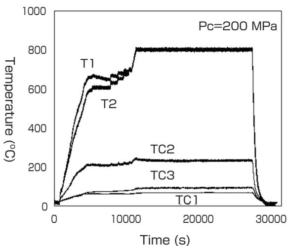
**Fig. 10 Performance test results of the developed heater<sup>[19]</sup>**
