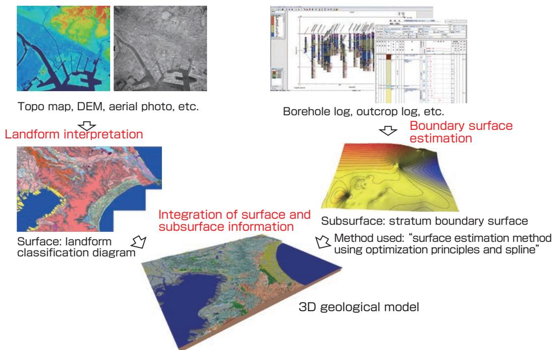
Fig. 5 Procedure of 3D modeling
