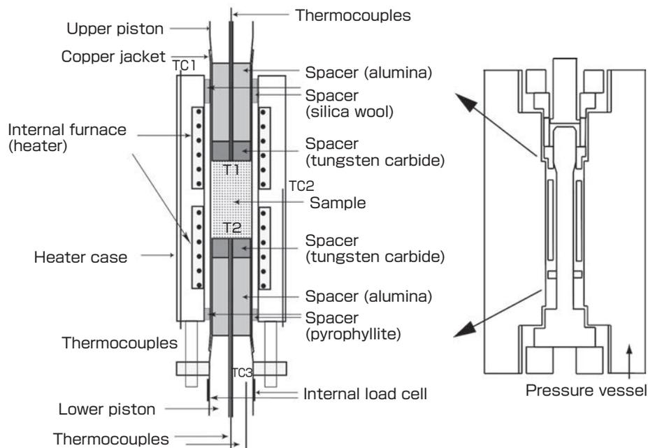
**Fig. 7 Schematic diagram of the pressure vessel<sup>[19]</sup>**
