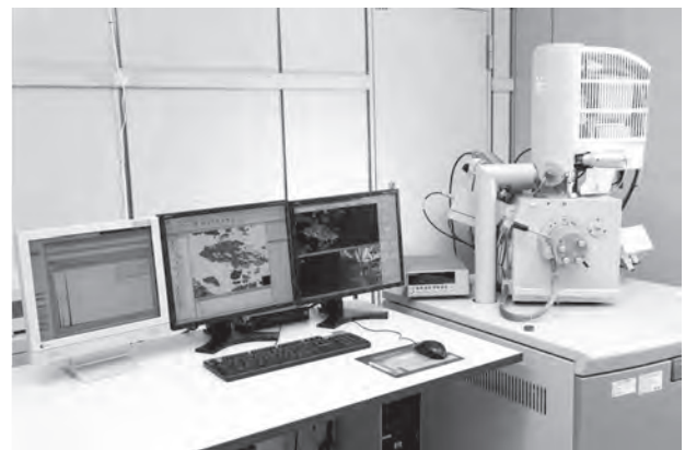
Fig. 6 Mineral liberation analyzer (MLA) by FEI
