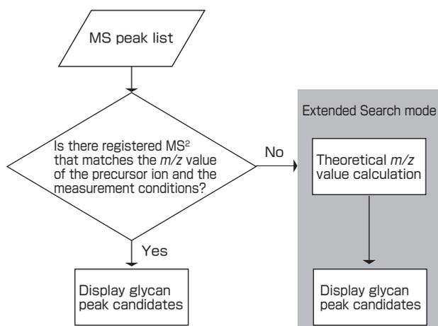
Fig. 5 Logic flow of the glycan peak detection
