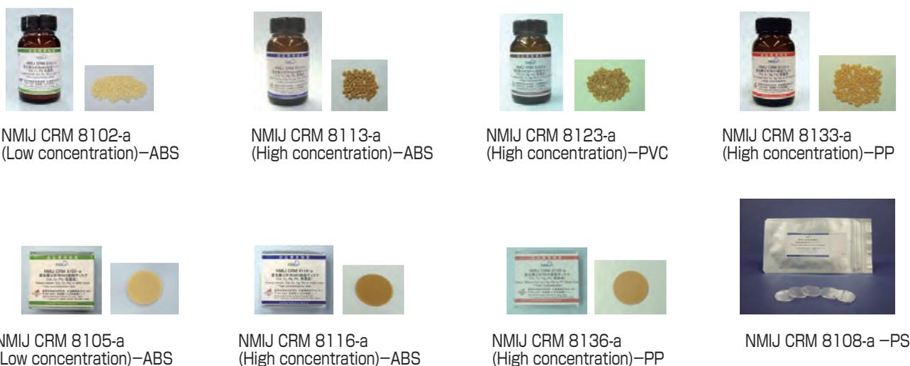
Fig. 7 Examples of the NMIJ CRMs in response to the RoHS directive
