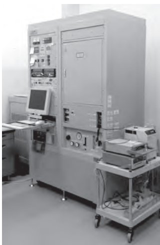
Fig. 7 The apparatus of national standard for thermal diffusivity
