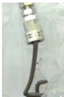
Fig. 5 Dewatered sludge supply by high-pressure sludge pump
