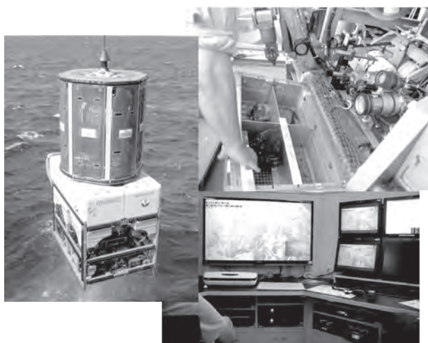
Fig. 7 Remotely operated vehicle (ROV) system on Hakurei, the vessel used for the GH12 cruise
