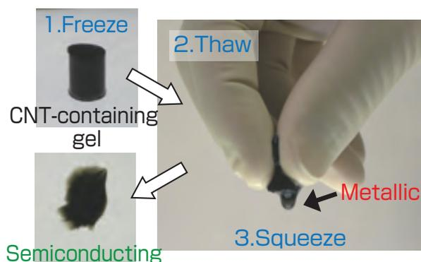
**Fig. 4 Separation of the metallic and semiconducting CNTs by freeze-thaw-squeeze method using the CNT-containing gel**
