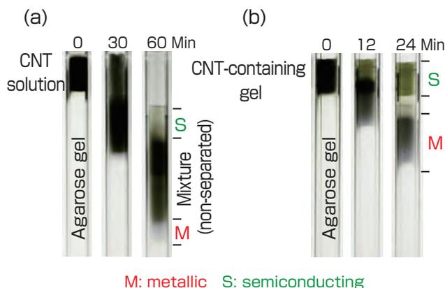
**Fig. 3 Separation of the metallic and semiconducting CNTs by agarose gel electrophoresis (a: solution sample, b: gel sample)**
