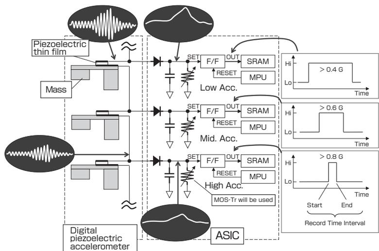
Fig. 5 Digital piezoelectric accelerometer
