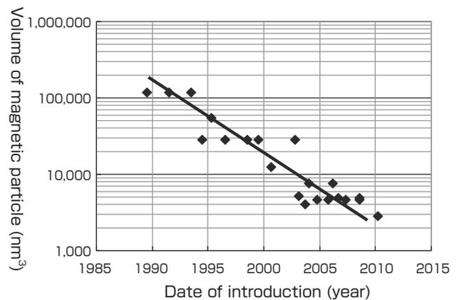
Fig. 3 Transition of the magnetic material volume
