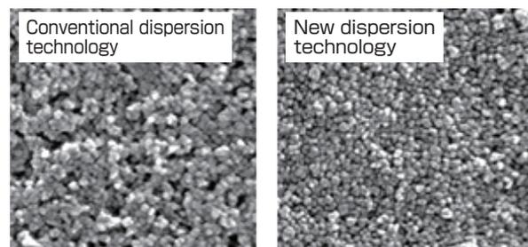
**Fig. 9 SEM image of the tape surface**
