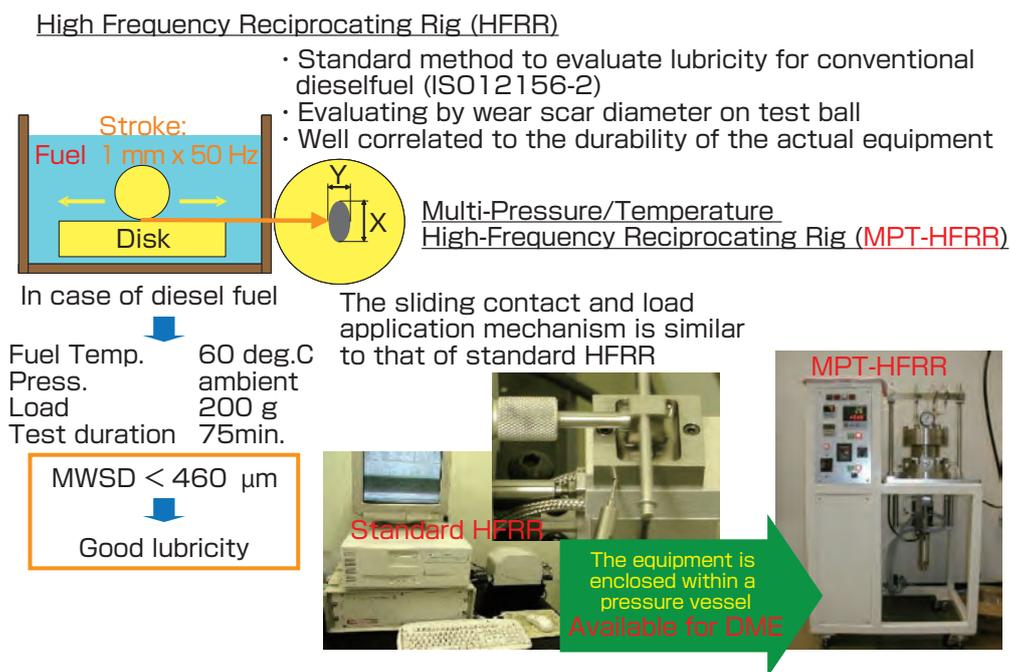
**Fig. 6 Lubricity evaluation device and evaluation method**
