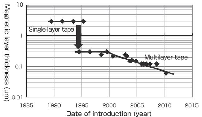
Fig. 4 Transition of the magnetic layer thickness<sup>[8][9]</sup>
