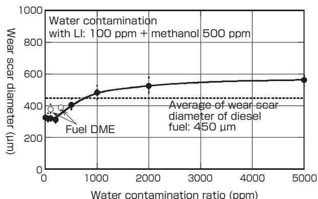
**Fig. 7 Effect of water contamination on abrasion scar diameter<sup>[1]\*</sup> (water 0–5,000 ppm, methanol 500 ppm)**
