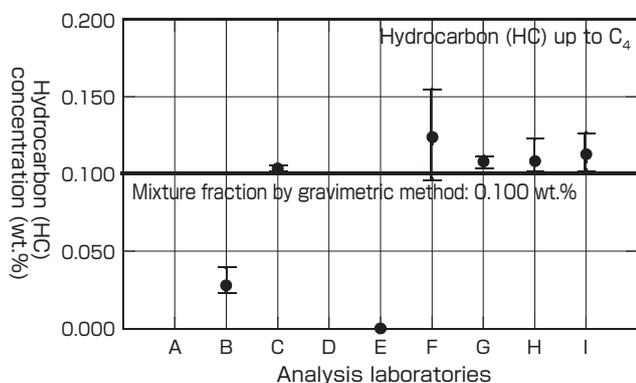
Fig. 9 Analysis result of hydrocarbon (HC) of C<sub>4</sub> or less in the round-robin test<sup>[9]\*</sup>
