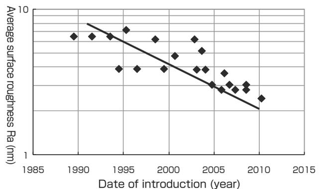
Fig. 5 Transition of the surface smoothness of tape
