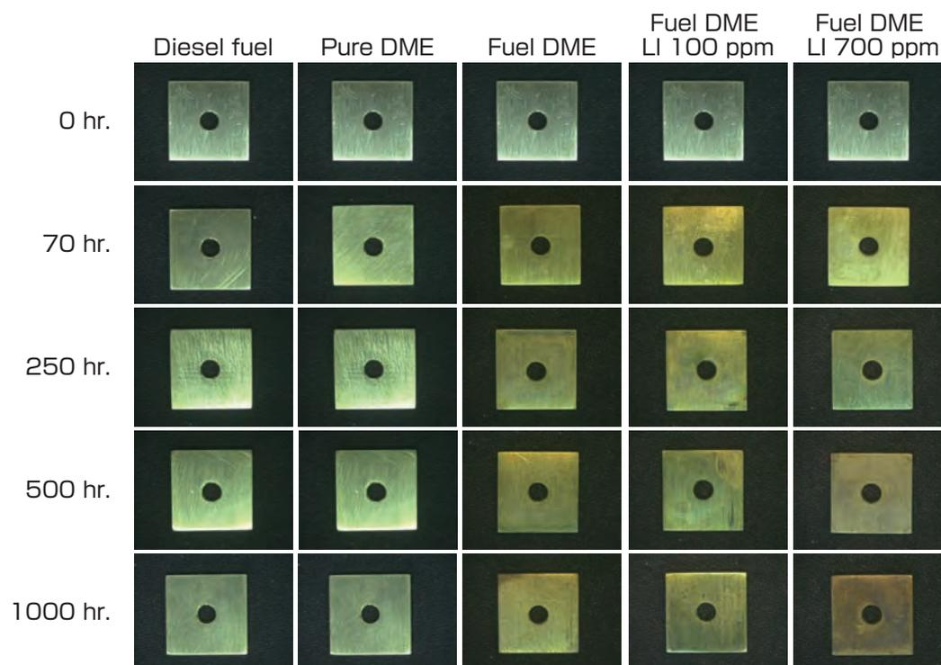
Fig. 4 Appearance of test piece after immersion test (brass C3604)<sup>[1]</sup>
