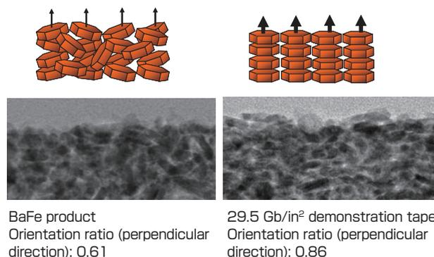
**Fig. 14 TEM image of the cross-section of magnetic layer<sup>[21]</sup>**
