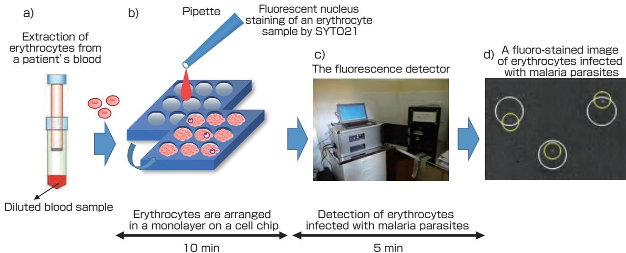
**Fig. 4 Workflow of the detection of erythrocytes infected with malaria parasites, using the cell chip<sup>[8]</sup>**
