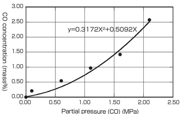
Fig. 13 Effect of CO partial pressure on CO solubility in DME<sup>[9]</sup>
