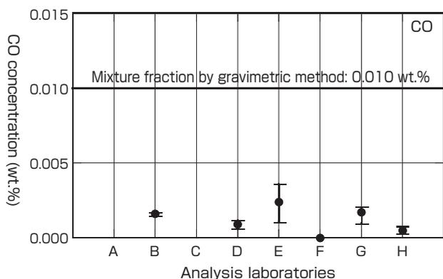
Fig. 11 Analysis result of carbon monoxide (CO) in the round-robin test<sup>[9]\*</sup>
