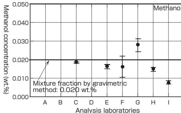
Fig. 10 Analysis result of methanol in the round-robin test<sup>[9]\*</sup>
