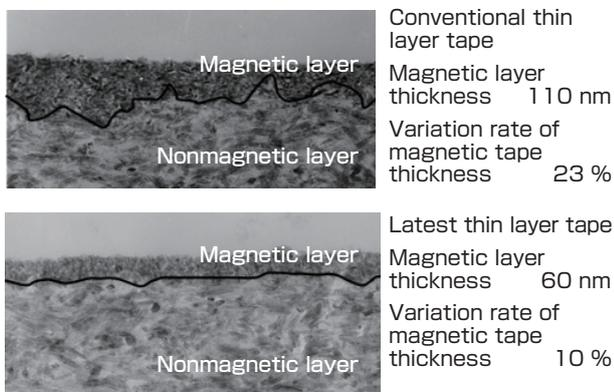
Fig. 10 TEM image of the tape cross-section
