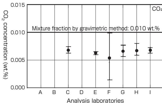
Fig. 12 Analysis result of carbon dioxide (CO<sub>2</sub>) in the round-robin test<sup>[9]\*</sup>
