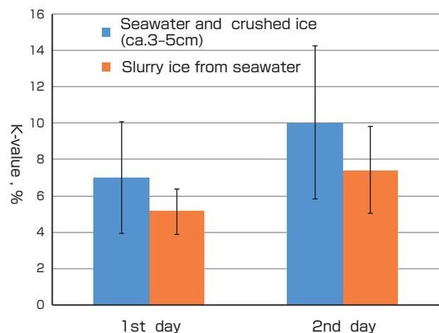
**Fig. 6 Comparison of K-values for two different cooling methods**
