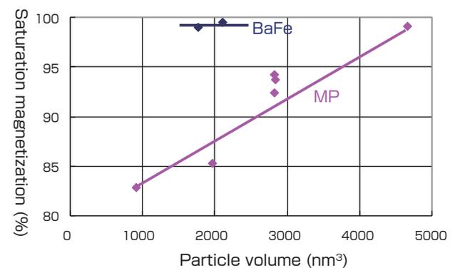
**Fig. 7 Change in the saturation magnetization (Ms) for one month storage at 60 °C and 90 % RH (relative humidity)**
