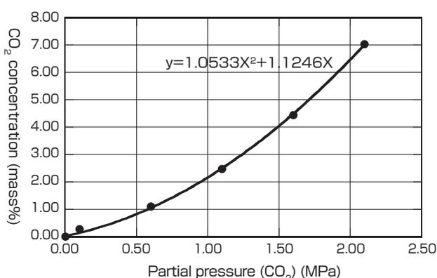
Fig. 14 Effect of CO<sub>2</sub> partial pressure on CO<sub>2</sub> solubility in DME<sup>[9]</sup>
