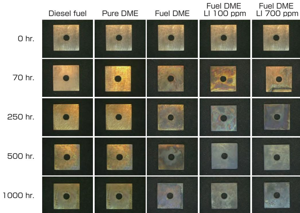
Fig. 3 Appearance of test piece after immersion test (Copper C1100)<sup>[1]</sup>
