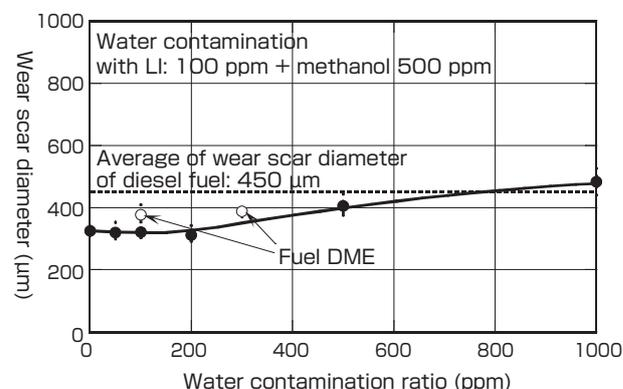
**Fig. 8 Effect of water contamination on abrasion scar diameter<sup>[1]\*</sup> (water 0–1,000 ppm, methanol 500 ppm)**
