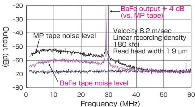
Fig. 11 Modulation spectra of the MP medium and the BaFe medium<sup>[10]</sup>
