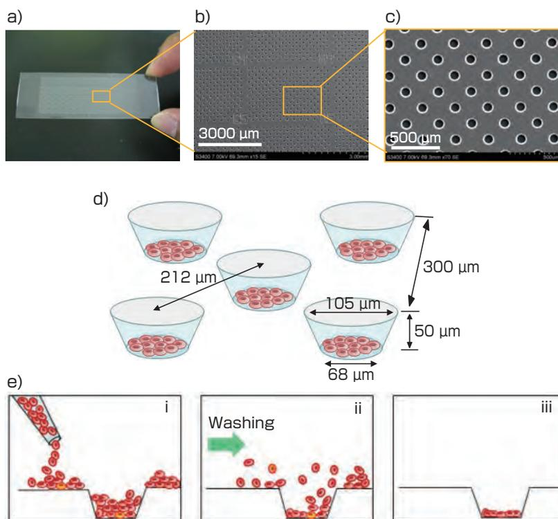
**Fig. 2 Structure of the cell chip and single layering of erythrocytes in the microchamber<sup>[8]</sup>**
