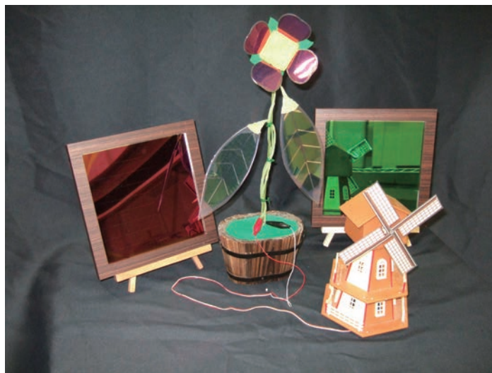
Various types of organic thin-film solar cell submodules providing excellent design flexibility This is produced through collaborative research with Mitsubishi Corporation and Tokki Corporation.
