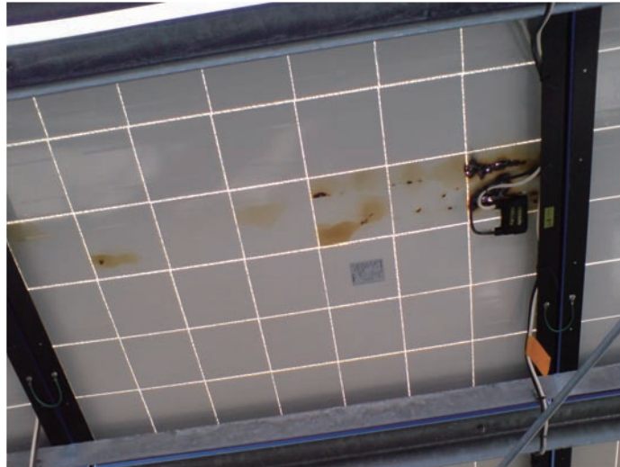
Example of a PV panel problem in AIST Mega-Solar Town at AIST Tsukuba The burned portion at the right was subjected to high temperature for several months.
