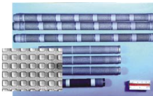
Fig. 1 SOFC (tubular type) developed by AIST, and electrode pattern on planar SOFC for ion dynamics analysis
