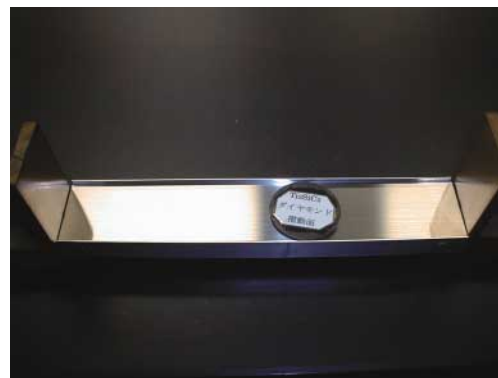
CVD diamond slider put on a stainless steel guide.
