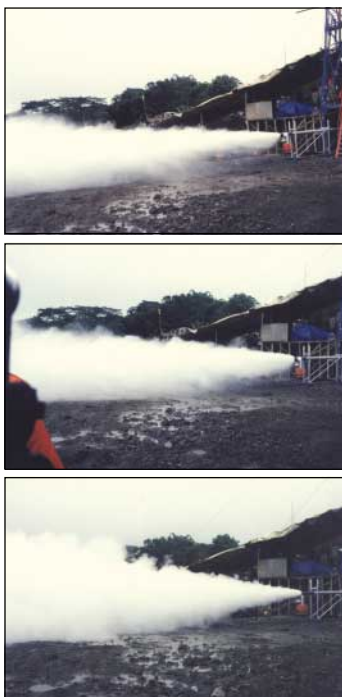
● Photo.1 (LEFT) Flow test of the NEDO geothermal exploration well on January 20, 2001
