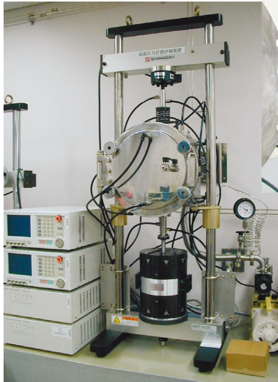
Photo : Experimental apparatus for evaluation of pressure sensors (Left: the whole apparatus; above: inside of the furnace)
