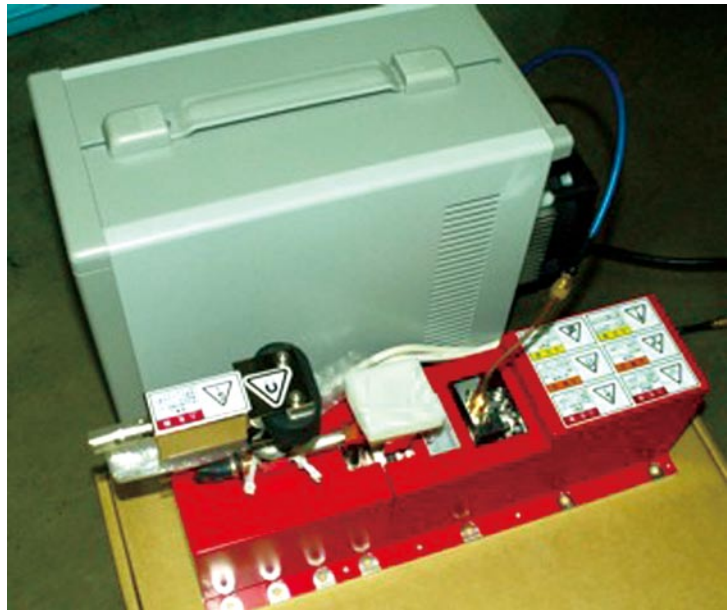
Photo 3. Microwave amplifier tube for X-band accelerator (front) and its driver unit (back)
