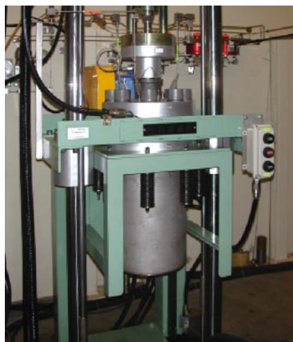
Hydrogen-gas embrittlement material-testing device
