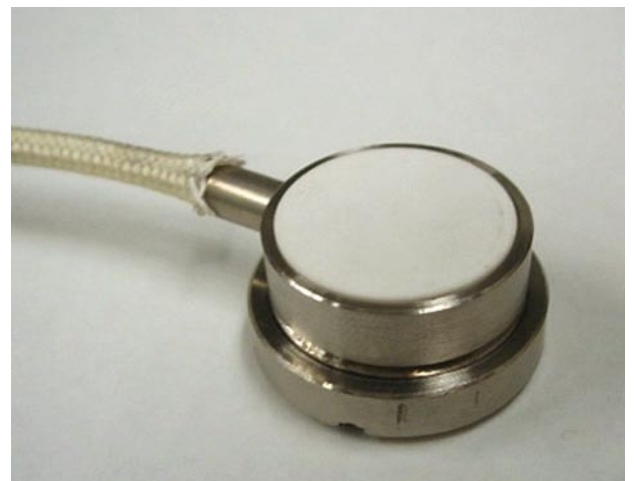
Figure 2. High-heat-resistant vibration AE sensor made of aluminum nitride (AlN)
