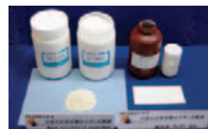
Fig.4 Visible-light-responsive \text{TiO}_2 photocatalysts. (left) powder, (right) Liquid for coating
