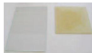
Fig.5 Thin-film photocatalyst coated on sheet glass. (left) \text{TiO}_2 , (right) Nitrogen-doped \text{TiO}_2 for visible-light activity
