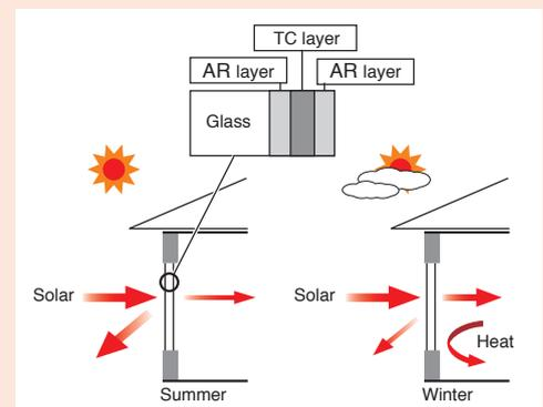
Schematic structure and performance of the window.
