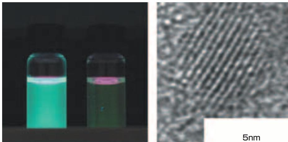
Fig. 3 ZnS/CdSe/ZnS nanoparticles (the left bottle) exhibit fluorescence at 480 nm with several dozen times stronger intensity than that of conventional CdSe/ZnS nanoparticles (the right bottle). The TEM image depicts the size of ZnS/CdSe/ZnS nanoparticles: ca. 5 nm diameter.
