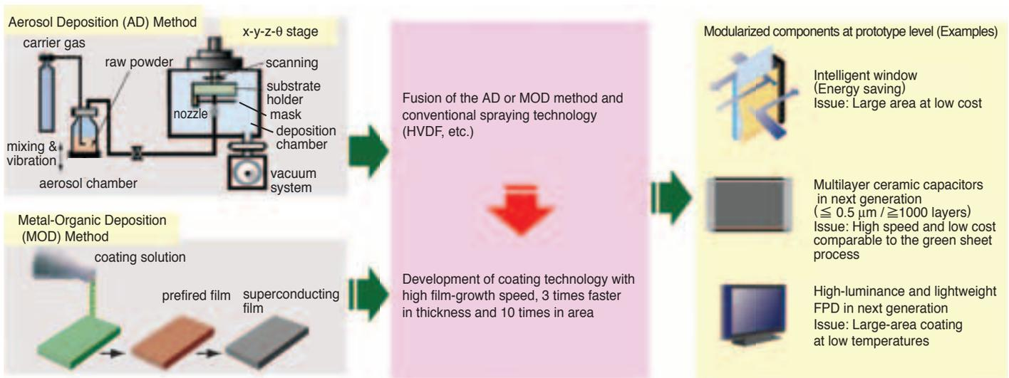
Fig. 2 Development of low-temperature and high-speed coating.
