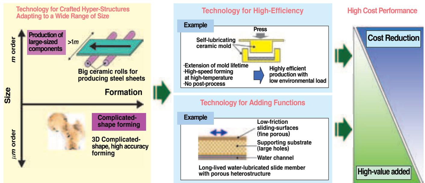
Fig. 3 Development of tailored manufacturing process.
