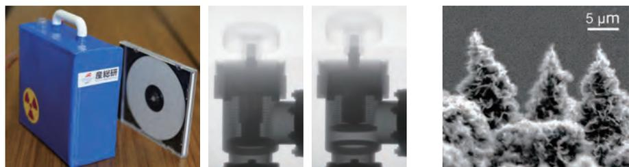
Picture (left figure) of the pulsed X-ray source compared with a CD case, and X-ray images (middle and right figures) of metallic valve at close and open positions
