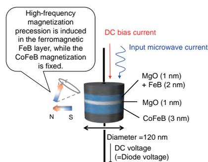
A schematic illustration of spin torque diode
