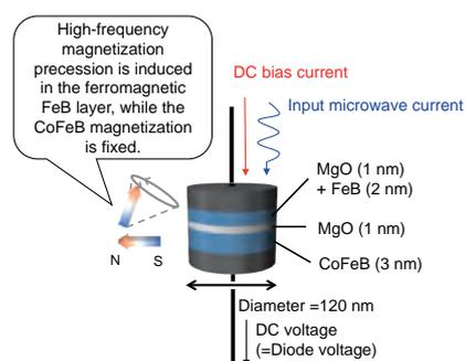
A schematic illustration of spin torque diode
