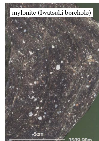
Figure : Photograph of polished slab of the mylonitic rock obtained from 3500m-deep Iwatsuki borehole.
