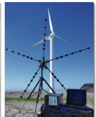
Noise measurement system
