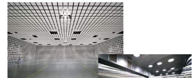
Electromagnetic Wave Anechoic Chamber
