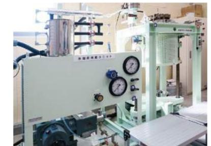
Experimental facility for the development of borehole tools for high-temperature and high-pressure geothermal wells
