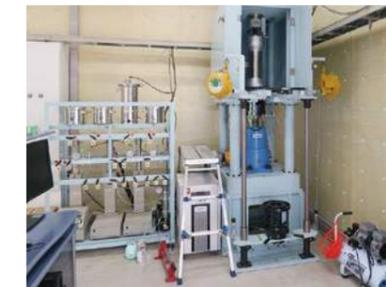
Experimental facility for shear slip of a fracture
