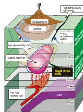
Concept of a supercritical geothermal system
