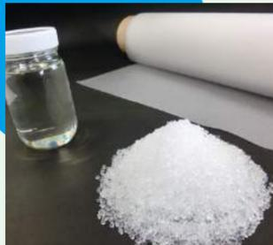
High-performance crosslinking coagent for EVA encapsulants in PV modules by Nippon Kasei Chemical Co., Ltd.
