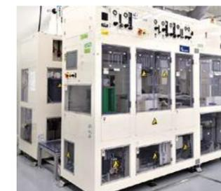
Spin etching apparatus
