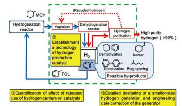
Fig. 1: Hydrogenation and dehydrogenation cycle of MCH
