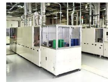
Electrode firing furnace
