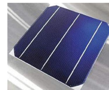
Crystalline silicon cell fabricated by standard FREA process
