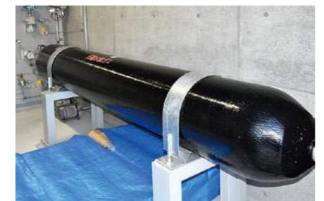
Fig. 2: High-pressure hydrogen device for fuel cell vehicle application development
