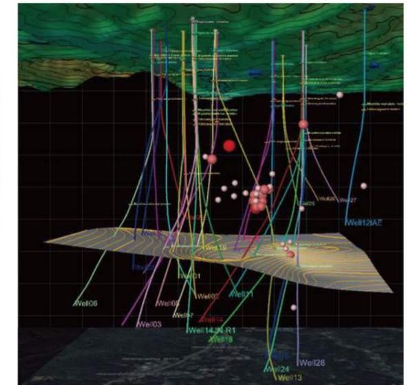
Microearthquake data integration and visualization system (monitoring the behavior of the injected water)
