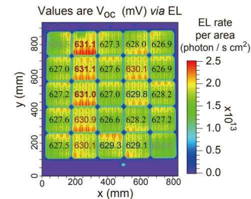
Voltage mapping using the absolute electroluminescence method
