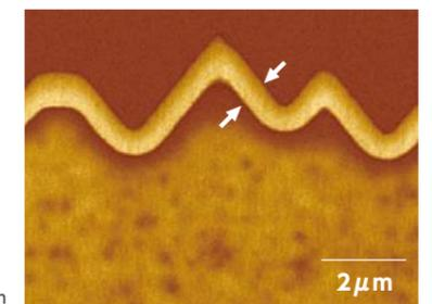
Phosphorus diffusion layer formed by ion implantation
