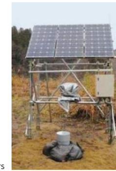
Installation status of three component seismometers
