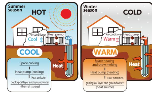
Concept of ground-source heat pump system
