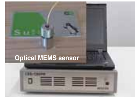
Multiplexing sensing instrument for optical MEMS sensor
